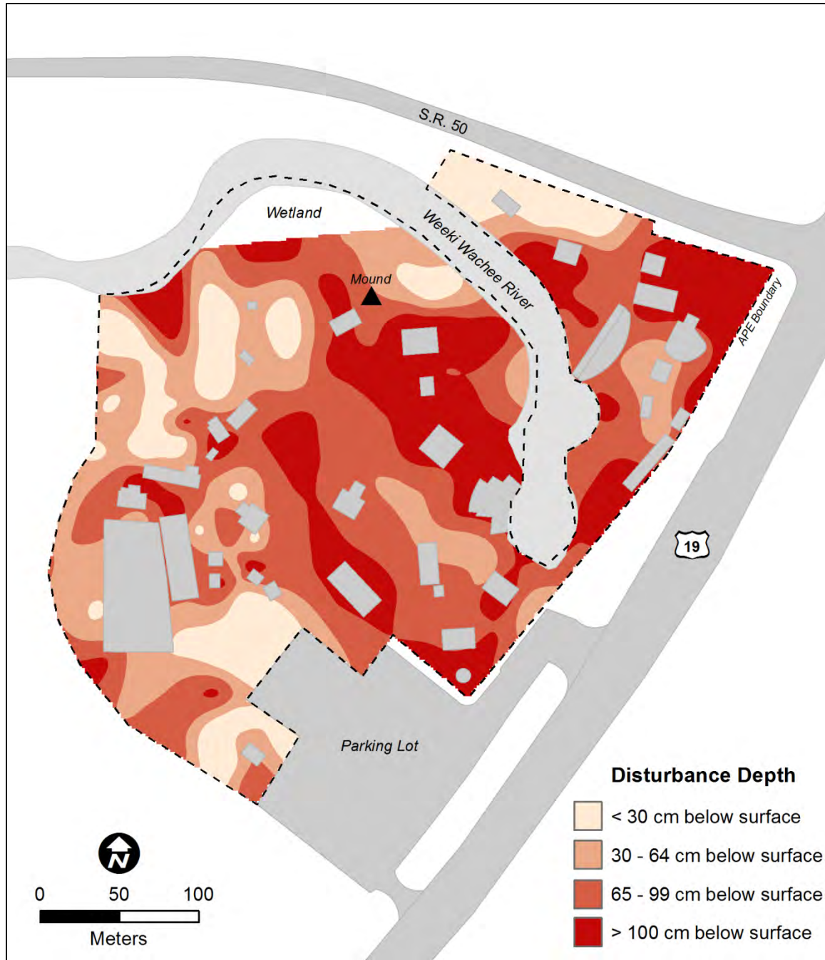
Figure 3-4. Interpolated depth of disturbance in the APE.
